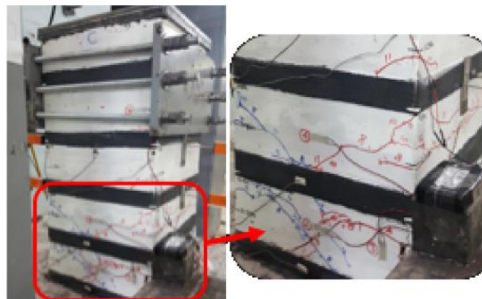
Fig. 8. A view of crack development measured with PZT.
