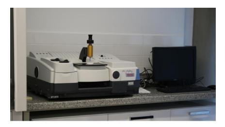
**Intended Use of the Instrument:** Chemical structure analysis of materials
